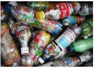
An **Ecobrick** is a plastic bottle packed to a set density with used, clean and dry plastic to achieve a building block that can be used over and over again. Ecobricks can also be packed with other non-biological un-recyclables that, uncontained, are toxic to the environment (i.e. styro-foam, wires, etc.).
