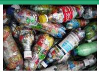
An **Ecobrick** is a plastic bottle packed to a set density with used, clean and dry plastic to achieve a building block that can be used over and over again. Ecobricks can also be packed with other non-biological un-recyclables that, uncontained, are toxic to the environment (i.e. styro-foam, wires, etc.).
